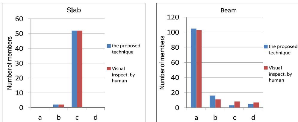
Figure 4.10: Comparison of the distribution of degradation levels obtained by diagnosis by human and the proposed technique
