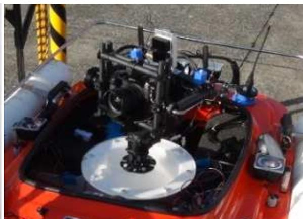
Figure 2.5: Photograph of the gimbal with image-shooting camera setup
