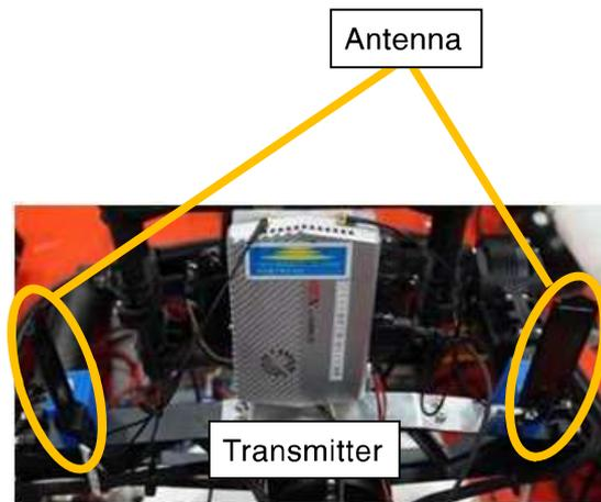
Figure 2.7: Transmitter for the camera by the image-shooting camera
