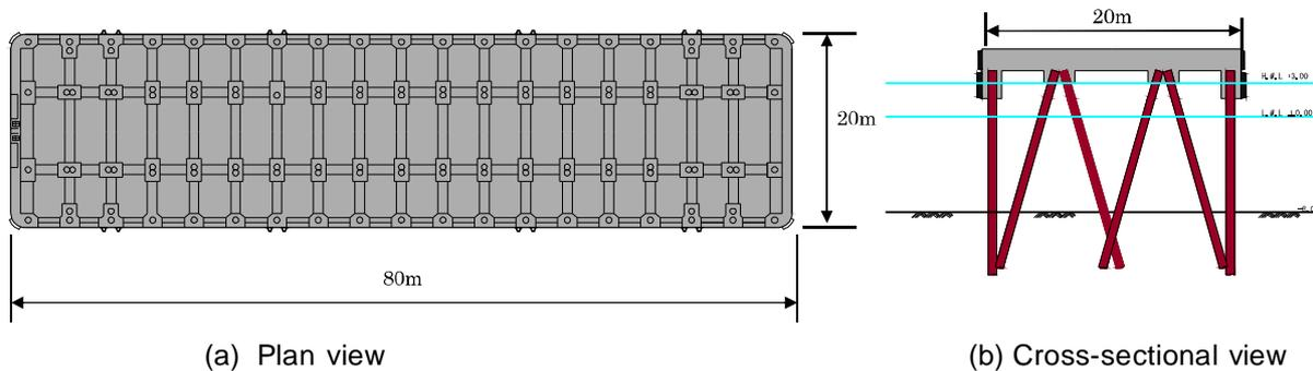
Figure 4.1: Plan view and cross-sectional view of a piled pier
