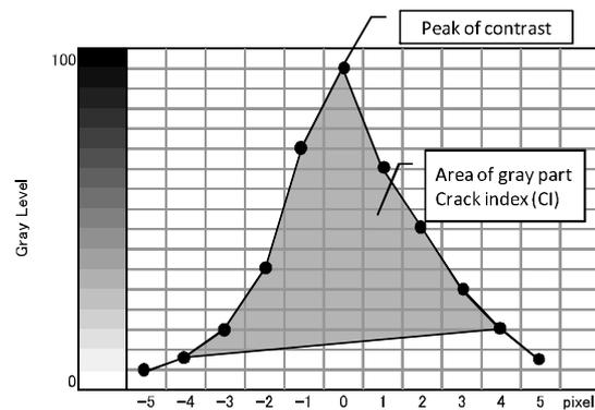
Figure 3.5: Crack width calculation method
