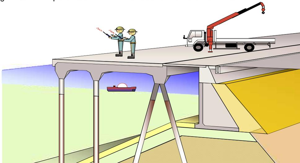
Figure 2.1: Inspection of the undersurface of the superstructure of a piled pier by an unmanned boat
