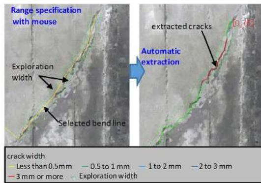
Figure 3.4: Image showing crack identification
