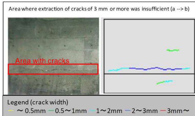
Figure 4.11: An area with different degrees of degradation
