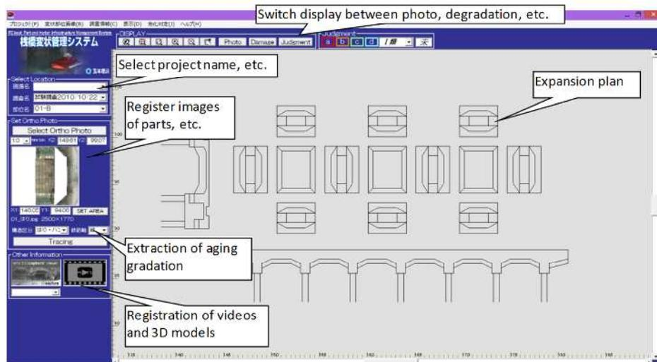
Figure 3.3: Main screen of the developed system
