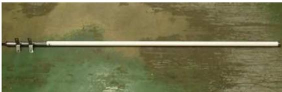
Figure 2.12: Transmission antenna of the emergency radio
