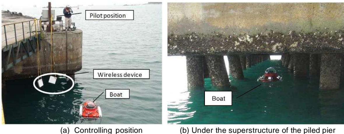
Figure 4.2: Trial test conducted on the undersurface of the superstructure of the piled pier
