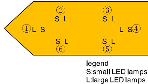
Figure 2.15: Diagrammatic arrangement of LED-lamps
