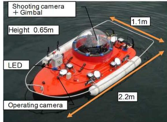
Figure 2.3: Unmanned boat (after mounting the devices)
