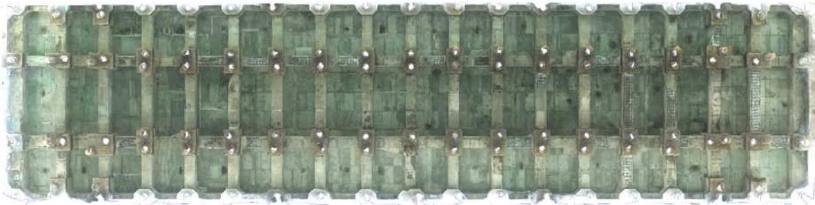
Figure 4.4: 3-D model of the undersurface of the superstructure of the piled pier (far view)
