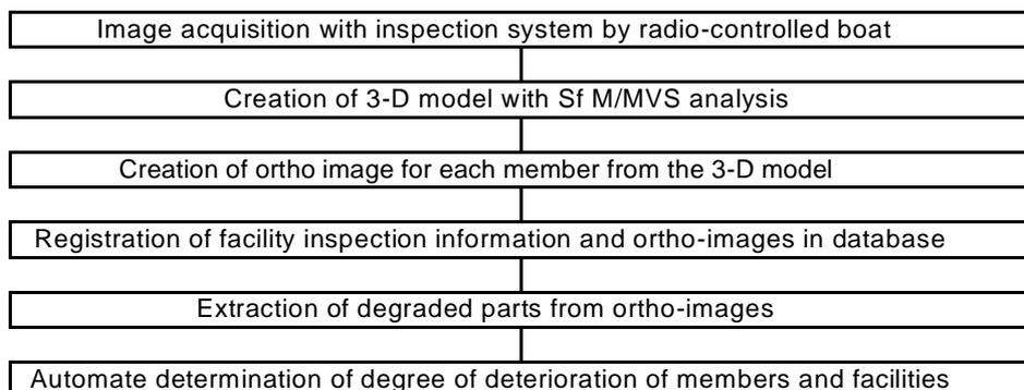
Figure 3.1: Flow-chart of data processing for automatic diagnosis of degradation
