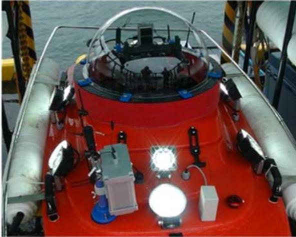
Figure 2.14: LED-lamps when active
