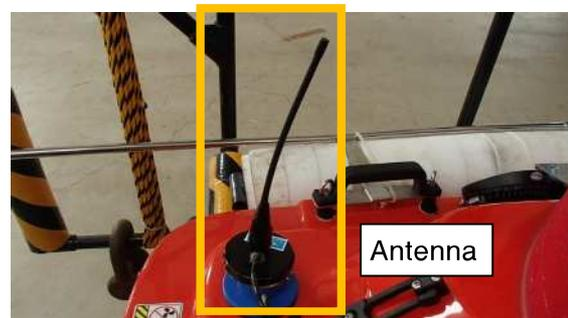
Figure 2.13: Reception antenna of the emergency radio
